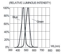
FIG.4 RELATIVE LUMINOUS INTENSITY VS. WAVELENGTH.
