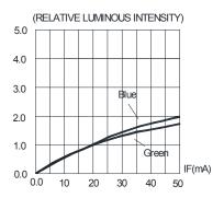
FIG.2 RELATIVE LUMINOUS INTENSITY VS. FORWARD CURRENT
