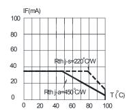
FIG.3 Green MAXIMUM FORWARD DC CURRENT VS AMBIENT TEMPERATURE (Tjmax=110 °C)
